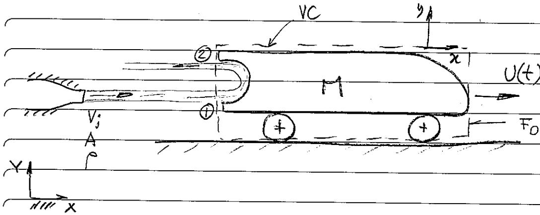
eq quant. mov. linear, dir x:  $F_x + F_{Bx} - \int_{Vc} a_{fx} pdA = \frac{\partial}{\partial t} \int_{Vc} u_{xyz} p dV + \int_{Vc} u_{xyz} p \vec{V}_{xyz} \cdot \vec{dA}$
