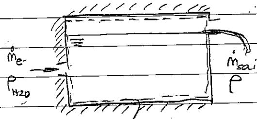
$$\text{eq. básica: } 0 = \frac{\partial}{\partial t} \int_{V_0} f dV + \int_{S_C} p \vec{V} \cdot d\vec{A}$$
